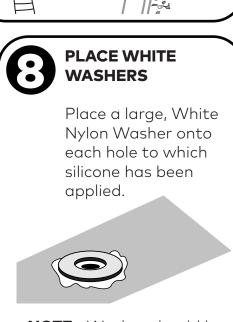
**NOTE -** Washer should be flat against drilled hole.
