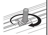
Twist Bolt assembly clockwise to engage with the track
