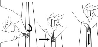
Insert Bolt by angling in and straightening
