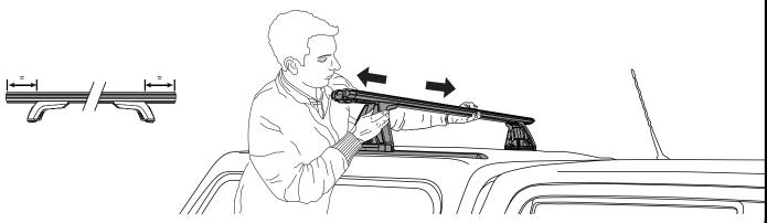
NOTE - Front and Rear Bars require individual adjustment due to tapered roof. Bars must be installed perpendicular to Tracks.
