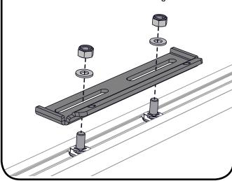
From the Gutter Mount Kit, position Nut Plates over holes on top of Legs.
