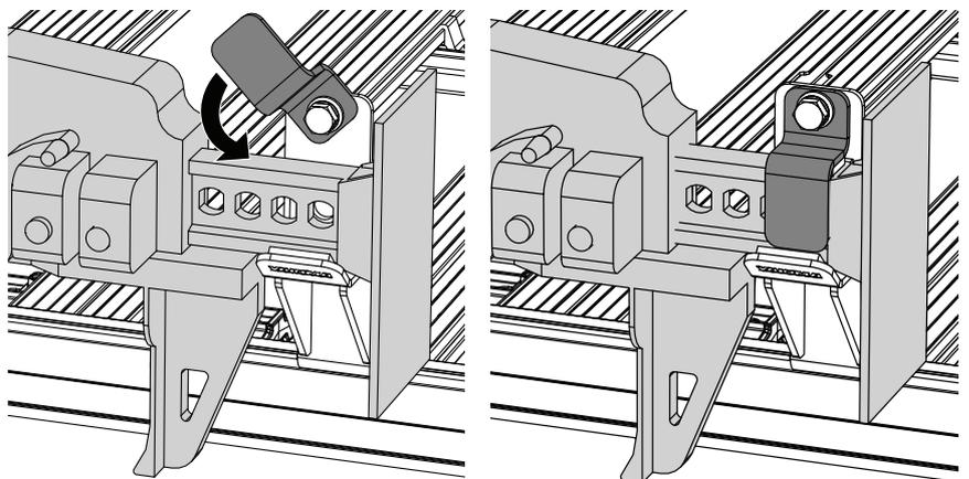
The jack can be secured with a padlock (not supplied) as shown for added security.
