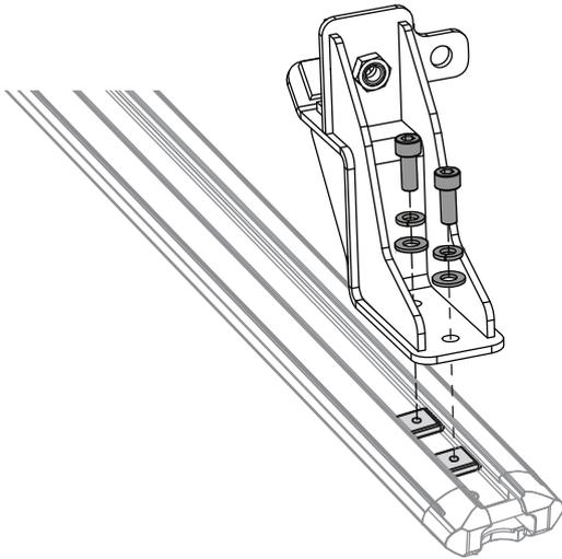
**SECURE BRACKETS - LockNLoad BAR**
