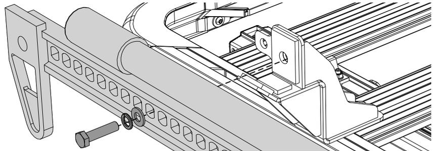
With the high lift jack securely in place, swing the clamp down over the jack arm and tighten the M10 x 30 mm Hex Screw.
