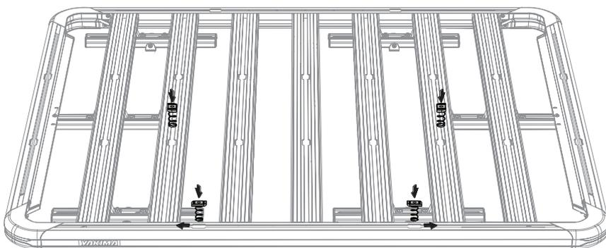
The Spring Nuts do not need to be rotated into place.
