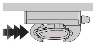
**Clamp must be seated correctly on crossbars, to avoid awning movement.**
