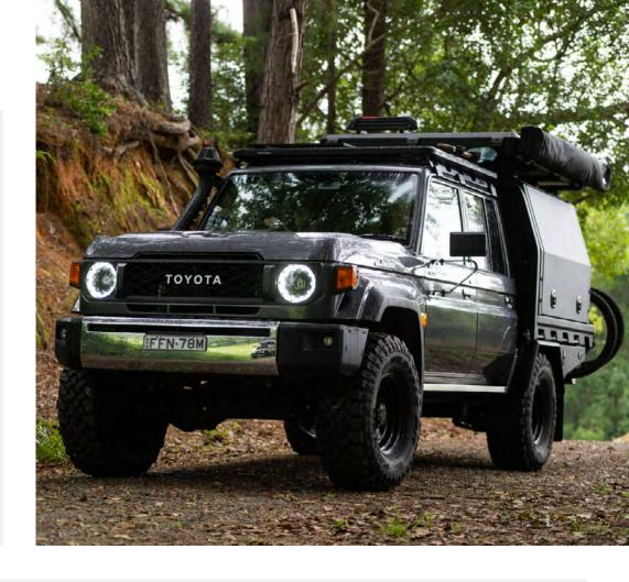
To calculate your maximum <u>offroad</u> capacity, first, subtract the <u>roof carrying solution + carrying accessory total weight</u> to your maximum on-road capacity. After that, subtract the offroad reduction percentage.
